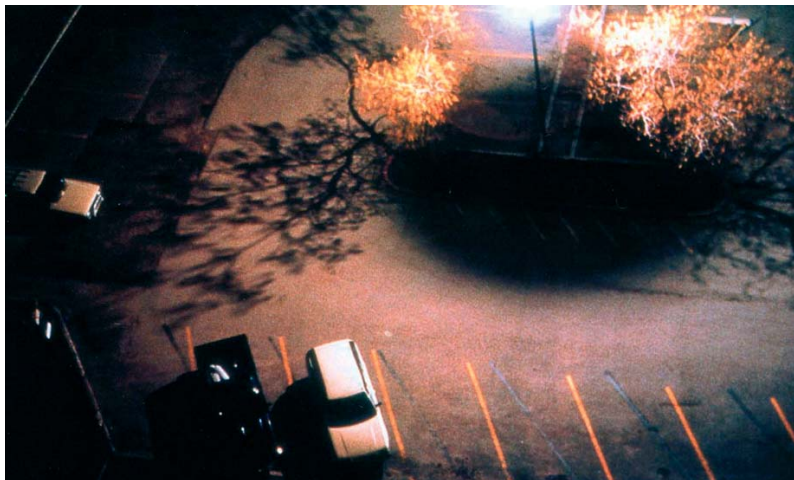
Globe lights fail to light the area below, spilling light sideways and upwards
